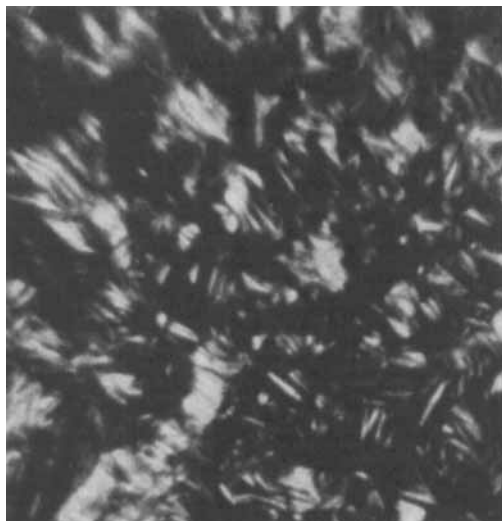
FIGURE 2 Micrograph of the hexagonal phase texture in SDS-water system (50% w/w) taken at 75 °C (indicated by A in Figure 1). See Color Plate I.
